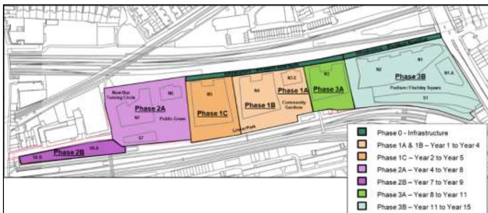
Figure 5.2: Indicative Construction Phasing Plan (note that Year 0 is assumed as 2022)
